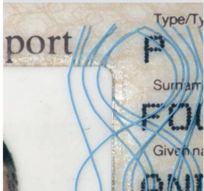
Intaglio printing in IR absorption
