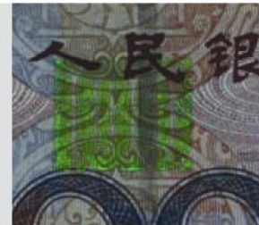
■ IR 740 - 1100 nm illumination for «Anti-stokes inks» examination
