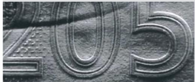
Intaglio printing in IR absorption
